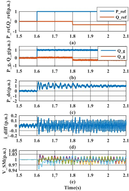
Fig. 8 (a) active and reactive reference (b) measured active and reactive power at grid bus (c) active power transferred to DC side (d) circulating current (e) SM capacitor voltages in upper arm of phase A
