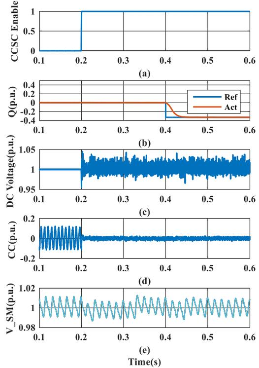
Fig. 7 (a) enable signal of CCSC (b) reactive power and reference value (c) DC bus voltage (d) circulating current (e) SM capacitor voltages in upper arm of phase A
