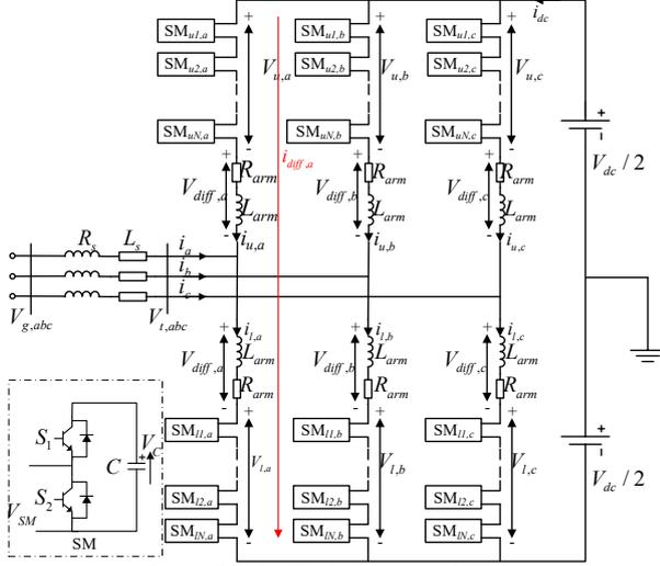
Fig. 1 The detailed diagram of MMC
