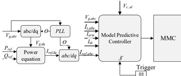
Fig. 4 Overall control Scheme of *M4*
