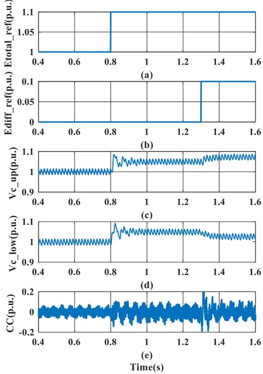
Fig. 6 (a) reference for total energy control (b) reference for balance control (c) upper arm capacitor voltages (d) lower arm capacitor voltages (e) circulating current
