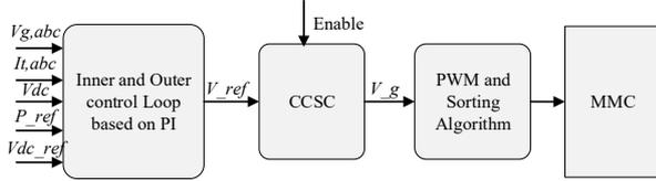
Fig. 3 Overall control Scheme of *M3*
