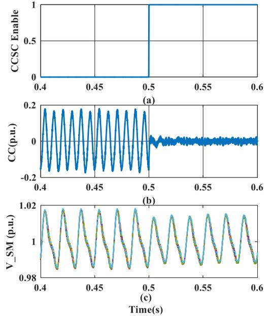
Fig. 5 (a) enable signal of CCSC; (b) circulating current (c) the capacitor voltages of phase A
