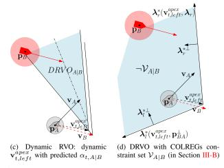
Fig. 1: Illustration of VO, RVO, DRVO and COLREGs constraints.
