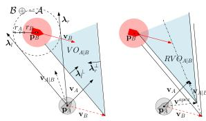
(a) Velocity obstacles (VO): colli- (b) Reciprocal VO: fixed  $\mathbf{v}^{apex} =$ sion cone  $CC_{A|B}$  translated by  $\mathbf{v}_B$
