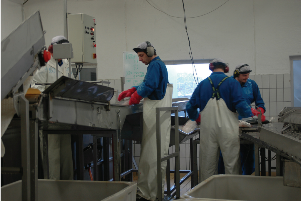
Figure 3.2 Manual grading and sorting of whole salmon in quality classes by human inspectors. Two to four persons per shift are necessary to carry out the task (Courtesy of Salmar AS).
