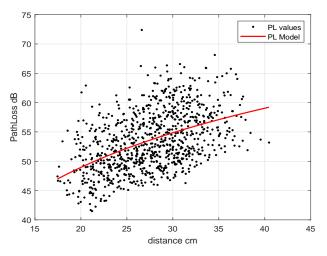
Figure 12. Path-loss eavesdropper link (IB2OFF, ISM).
