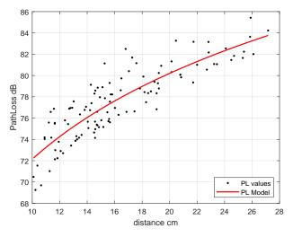
Figure 14. Path-loss Eve link without blood (IB2OFF UWB).
