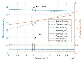
Figure 3. Dielectric Properties of ISM Phantom.
