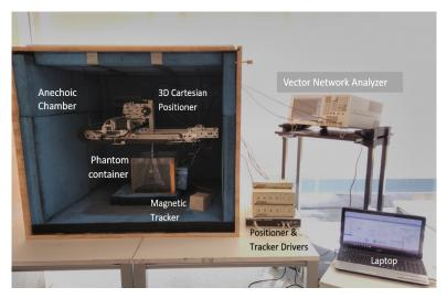
Figure 2. Measurement Setup.
