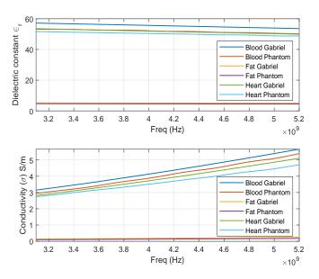
Figure 6. Dielectric Properties of UWB Phantom.
