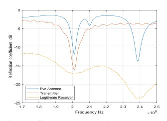
Figure 4. Reflection coefficients for Legitimate and Eavesdropper antennas (ISM).
