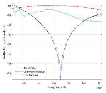
Figure 8. S-parameters of UWB antennas.
