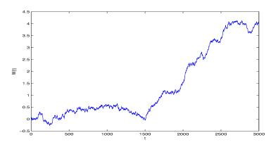
Figure 5.1.1: Piecewise Wiener process simulated in the time interval  $[0, t_n] = [0, 3000]$ . with one change point  $\tau = 1500$ . The drift parameter before the change point is  $\nu_0 = 0$ and after the change point  $\nu = 0.003$ . The variance parameter is the same for both pieces,  $\sigma = 0.02$ . For this process, we will consider the threshold a = 14.
