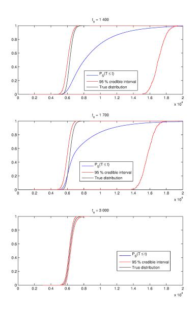
Figure 5.1.6: Simulation approach to estimating CDF,  $\hat{P}_S(T \leq t)$  for different observation lengths,  $t_n$ , shown with 95 % credible intervals and the true distribution. The *x*-axis is time *t* while the *y*-axis is the probability. Top panel:  $t_n = 1$  400. Middle panel:  $t_n = 1$  700. Bottom panel:  $t_n = 3$  000. Here,  $\nu$  and  $\sigma$  are considered known parameters, while  $\tau$  is unknown.
