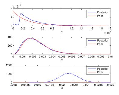
Figure 5.1.14: Prior distributions of  $\tau$ ,  $\pi(\tau)$ ,  $\nu$ ,  $\pi(\nu)$  and  $\sigma$ ,  $\pi(\sigma)$  and posterior distribution of  $\tau$ ,  $\pi(\tau|x_1, \ldots, x_n; \nu, \sigma)$ ,  $\nu$ ,  $\pi(\nu|x_1, \ldots, x_n; \nu, \sigma)$  and  $\sigma$ ,  $\pi(\sigma|x_1, \ldots, x_n; \nu, \sigma)$  given the observed temperature W(t) up until  $t_n = 1$  400. Here,  $\tau$ ,  $\nu$  and  $\sigma$  were considered unknown.
