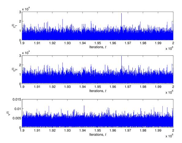
Figure A.2.17: Trace plot of the last 100 000 iterations of the Markov chain from the marginal posterior distributions of  $\tau_1, \pi(\tau_1|x_1, \ldots, x_n; \alpha, \sigma), \tau_2, \pi(\tau_2|x_1, \ldots, x_n; \alpha, \sigma)$  and  $\nu, \pi(\nu|x_1, \ldots, x_n; \alpha, \sigma)$ . Here,  $\sigma$  and  $\alpha$  were considered known, and the endpoint of observations was  $t_n = 700$ .
