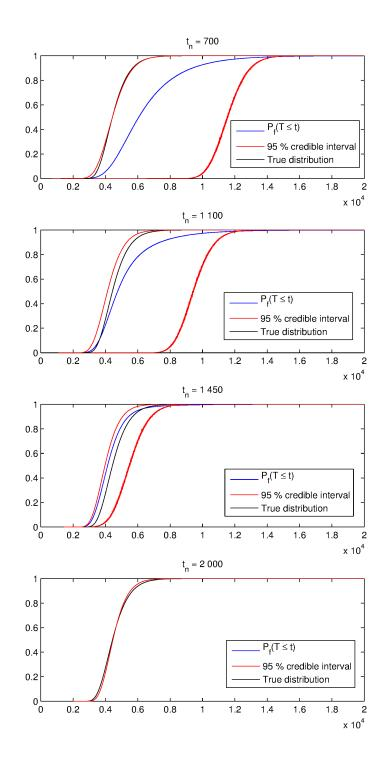
Figure 5.2.6: Formulaic approach to estimating CDF,  $\hat{P}_f(T \leq t)$  shown with 95 % credible intervals for different observation lengths,  $t_n$ . Shown with true distribution. Here,  $\tau_1$  and  $\tau_2$  are unknown parameters,  $\nu$ ,  $\sigma$  and  $\alpha$  are known parameters. Top panel:  $t_n = 700$ . Second panel:  $t_n = 1$  100. Third panel:  $t_n = 1$  450. Bottom panel:  $t_n = 2$  000. The x-axis is time and y-axis is probability.
