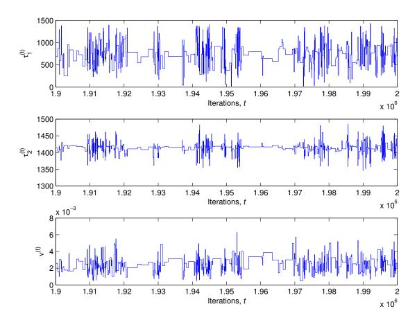
Figure A.2.29: Trace plot of the last 100 000 iterations of the Markov chain from the marginal posterior distributions of  $\tau_1, \pi(\tau_1|x_1, \ldots, x_n; \alpha, \sigma), \tau_2, \pi(\tau_2|x_1, \ldots, x_n; \alpha, \sigma)$  and  $\nu, \pi(\nu|x_1, \ldots, x_n; \alpha, \sigma)$ . Here,  $\sigma$  and  $\alpha$  were considered known, and the endpoint of observations was  $t_n = 2$  000.
