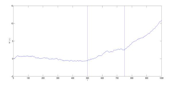
Figure 4.1.2: A realization of a Wiener process in the time interval [0, 1000] with two change points:  $\tau_1 = 500, \tau_2 = 750$ , marked with vertical lines. The process was simulated with the following parameters:  $\nu_0 = 0, \nu_1 = 0.015, \nu_2 = 0.035$  and  $\sigma_i = \sigma = 0.05, i = 0, 1, 2$ .
