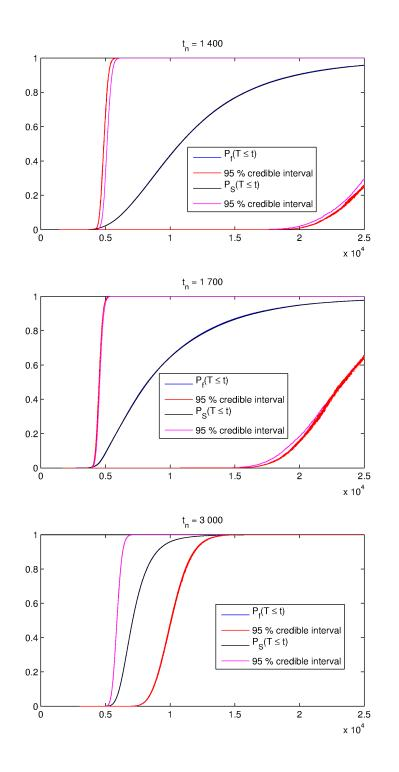
Figure 5.1.19: Comparison of the simulation and formulaic approaches,  $\hat{P}_S(T \leq t)$  and  $\hat{P}_f(T \leq t)$  with  $\tau$ ,  $\nu$  and  $\sigma$  as unknown parameters, for three different observation lengths  $t_n$ . Top panel:  $t_n = 1$  400. Middle panel:  $t_n = 1$  700. Bottom panel:  $t_n = 3$  000. The *x*-axis is time *t* while the *y*-axis is the probability.
