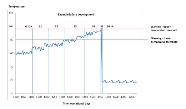
Figure 2.1.1: Example of a typical temperature process through failure development given in Valland et al. (2012). S1 denotes stage 1, S2 denotes state 2 and so on. Note that state 0 which has been added in this thesis corresponds to OK.
