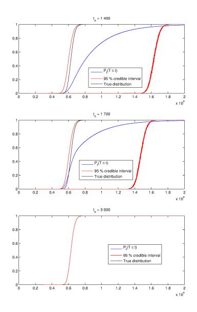
Figure 5.1.5: Formulaic approach to estimating CDF,  $\hat{P}_f(T \leq t)$  for different observation lengths,  $t_n$ , shown with 95 % credible intervals and the true distribution. The *x*-axis is time *t* while the *y*-axis is the probability. Top panel:  $t_n = 1$  400. Middle panel:  $t_n = 1$ 700. Bottom panel:  $t_n = 3$  000. Here,  $\nu$  and  $\sigma$  are considered known parameters, while  $\tau$  is unknown.
