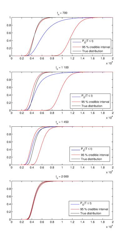
Figure 5.2.7: Simulation approach to estimating CDF,  $\hat{P}_S(T \leq t)$  shown with 95 % credible intervals for different observation lengths,  $t_n$ . Shown with true distribution. Here,  $\tau_1$  and  $\tau_2$  are unknown parameters,  $\nu$ ,  $\sigma$  and  $\alpha$  are known parameters. Top panel:  $t_n = 700$ . Second panel:  $t_n = 1$  100. Third panel:  $t_n = 1$  450. Bottom panel:  $t_n = 2$  000. The x-axis is time and y-axis is probability.
