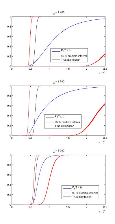
Figure 5.1.17: Formulaic approach to estimating CDF,  $\hat{P}_f(T \leq t)$  for different observation lengths,  $t_n$ , shown with 95 % credible intervals and the true distribution. The *x*-axis is time *t* while the *y*-axis is the probability. Top panel:  $t_n = 1$  400. Middle panel:  $t_n = 1$  700. Bottom panel:  $t_n = 3$  000. Here,  $\tau$ ,  $\nu$  and  $\sigma$  are unknown parameters.
