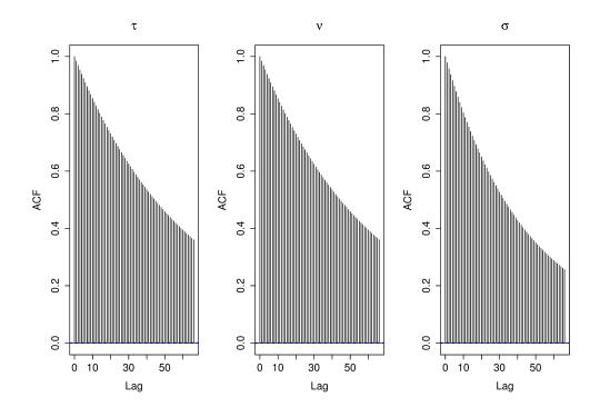
Figure A.1.25: Autocorrelation of the iterations in the Markov chain from the marginal posterior distributions of  $\tau$ ,  $\pi(\tau|x_1, \ldots, x_n)$ ,  $\nu$ ,  $\pi(\nu|x_1, \ldots, x_n)$  and  $\sigma$ ,  $\pi(\sigma|x_1, \ldots, x_n)$ , as function of the lag. The endpoint of observation was  $t_n = 1$  400.
