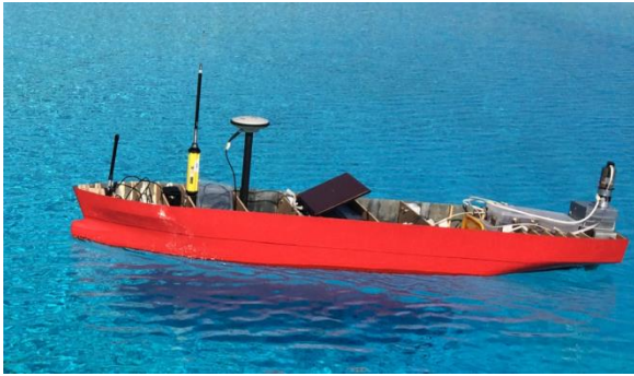
FIGURE 1: Scaled self-running ship model in the test.
