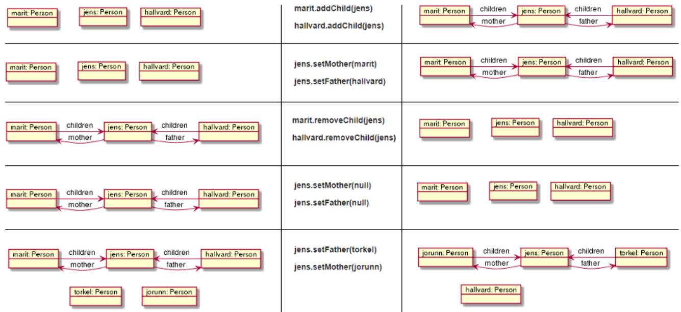
Figure 1. Consistencies absent from the original version of the code provided to participants in the present study. There were a few consistency checks implemented as unit tests. 1) Gender consistency: the mother should be female and the father should be male. 2) Child–parent consistency: if Jens is the child of Merit, Merit should be the mother of Jens, and vice-versa. 3) The removal of a child–parent relationship from either a parent or a child should also apply to the whole family. 4) Adoption consistency: the child–parent (addition and removal) and the gender consistencies should be maintained in the case of adoption.
