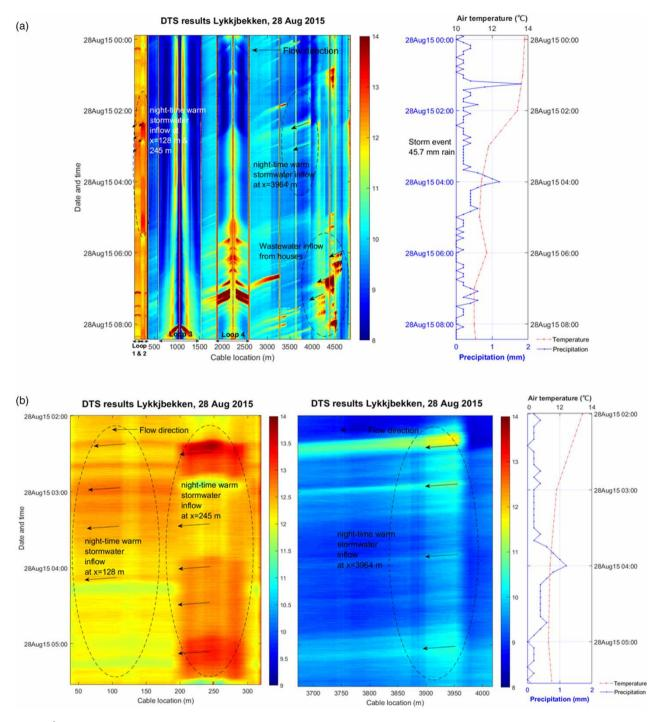
Figure 4 (a) DTS monitoring results in foul sewer network of Lykkjbekken catchment (left), with 5 min precipitation and hourly temperature data (right), 27–28 August, 2015, and (b) a closer view of rainfall-derived I/I at x = 128 m and 245 m (left) and x = 3,964 m (middle), with 5 min precipitation and hourly temperature data (right). Color-gradient scales indicate temperature (°C).
