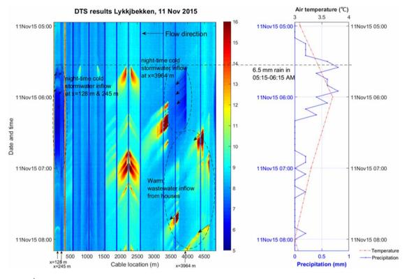
Figure 5 | DTS monitoring data in foul sewer network of Lykkjbekken catchment (left), with 5 min rainfall depth and hourly temperature data (right) for November 11, 2015. Color-gradient scales indicate temperature (°C).
