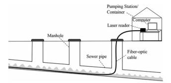
Figure 1 Schematic outline of the DTS method in a sewer pipe and the control unit stored outside the sewer system in the pumping station (Beheshti & Sægrov 2018a).
