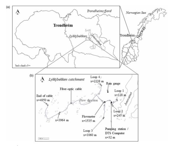
Figure 3 | (a) The location of Lykkjbekken catchment in Trondheim, Norway, (b) DTS cable installation in Lykkjbekken catchment.
