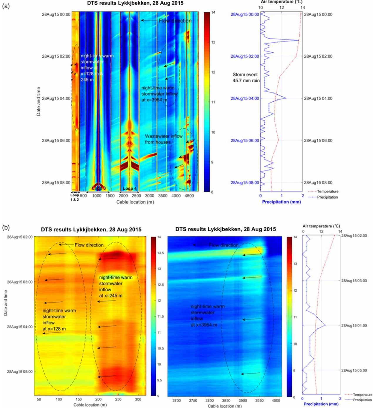
**Figure 4** | (a) DTS monitoring results in foul sewer network of Lykkjebekken catchment (left), with 5 min precipitation and hourly temperature data (right), 27–28 August, 2015, and (b) a closer view of rainfall-derived I/I at  $x = 128$  m and  $245$  m (left) and  $x = 3,964$  m (middle), with 5 min precipitation and hourly temperature data (right). Color-gradient scales indicate temperature ( $^{\circ}\text{C}$ ).
