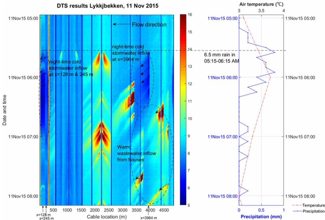
**Figure 5** | DTS monitoring data in foul sewer network of Lykkjebekken catchment (left), with 5 min rainfall depth and hourly temperature data (right) for November 11, 2015. Color-gradient scales indicate temperature ( $^{\circ}\text{C}$ ).
