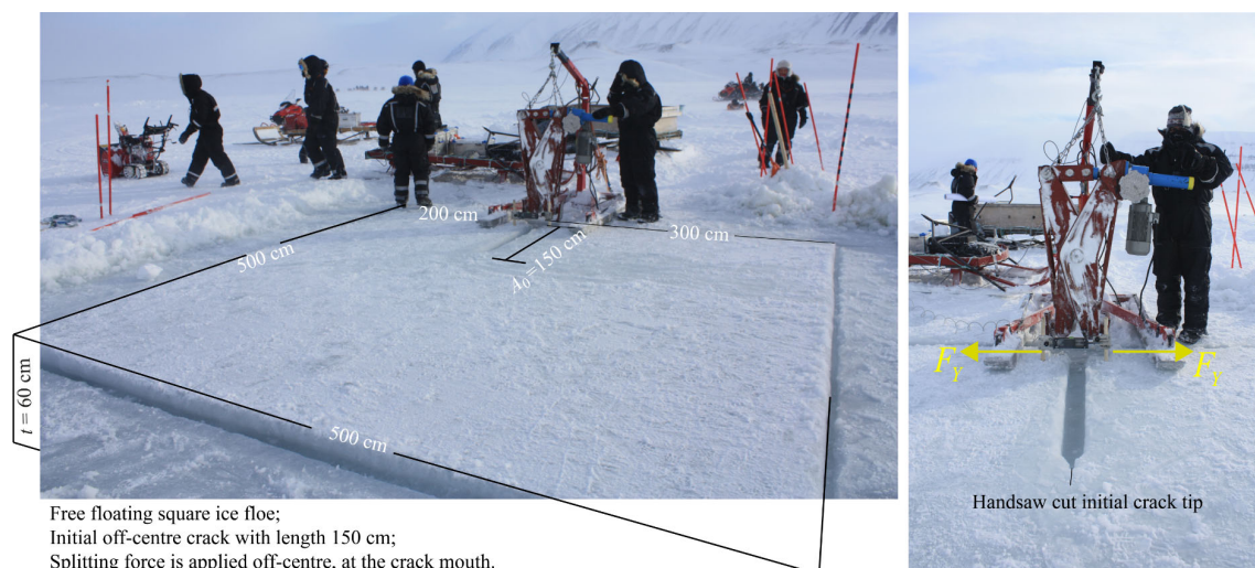
Fig. 12. Field off-centre splitting test set-up.
