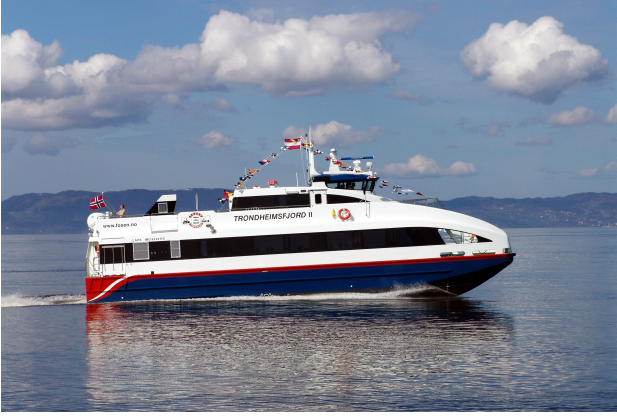
Fig. 2. The MS Trondheimsjord II is high-speed catamaran for passenger transport. Length 24.5 m, beam 8.0 m and maximum speed 16.5 m/s (32 knots).
