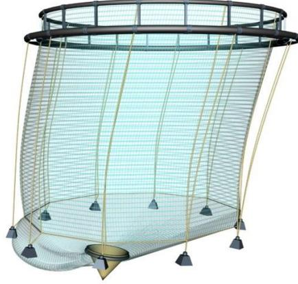
Figure 1: Floating fish farm with circular plastic collar consisting of two tori that are nearly semi-submerged in calm water, railing, jump net, netting, dead fish removal system, frame of ropes and bottom weights. (Sintef Fisheries and Aquaculture).
