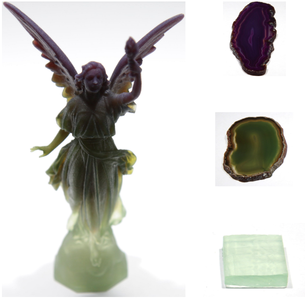
Fig. S3. The St. Lucy model printed (10cm) with varying RGBA values. At the top is that of the violet stone, middle is green stone and bottom is green soap, with linear transitions in between.
