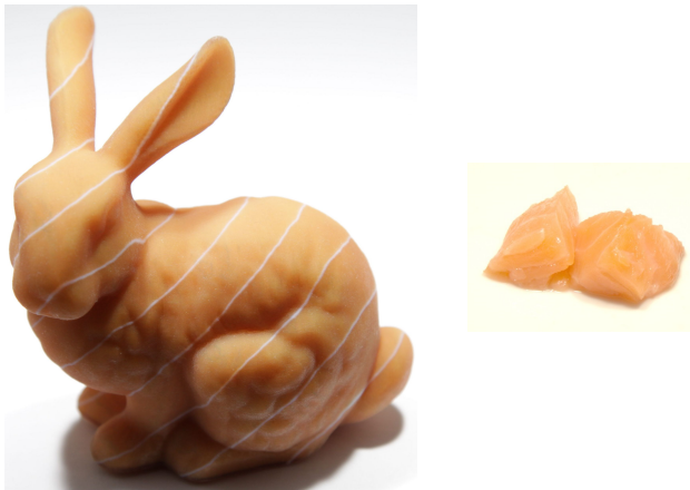
Fig. S4. The Stanford Bunny printed (10cm) with the measured RGBA values from the salmon. The white, opaque stripes are added procedurally.
