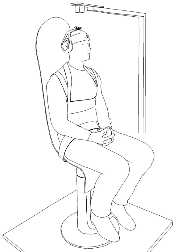
Figure 1. An instrumented participant strapped to the actuated chair. The cube above the persons' head represents the electromagnetic transmitter. Note that the ear muffs have holes leaving the ears uncovered and hearing intact (Stensdotter et al., Physiological Reports , 2016).
