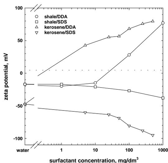
Fig. 3. Dependencies of zeta potential values of kerosene droplets and shale particles on ionic surfactant concentration
