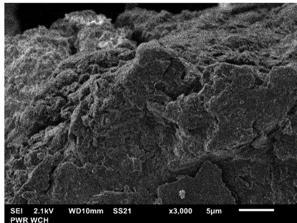
Fig. 1. SEM of shale originated from Kupferschiefer
