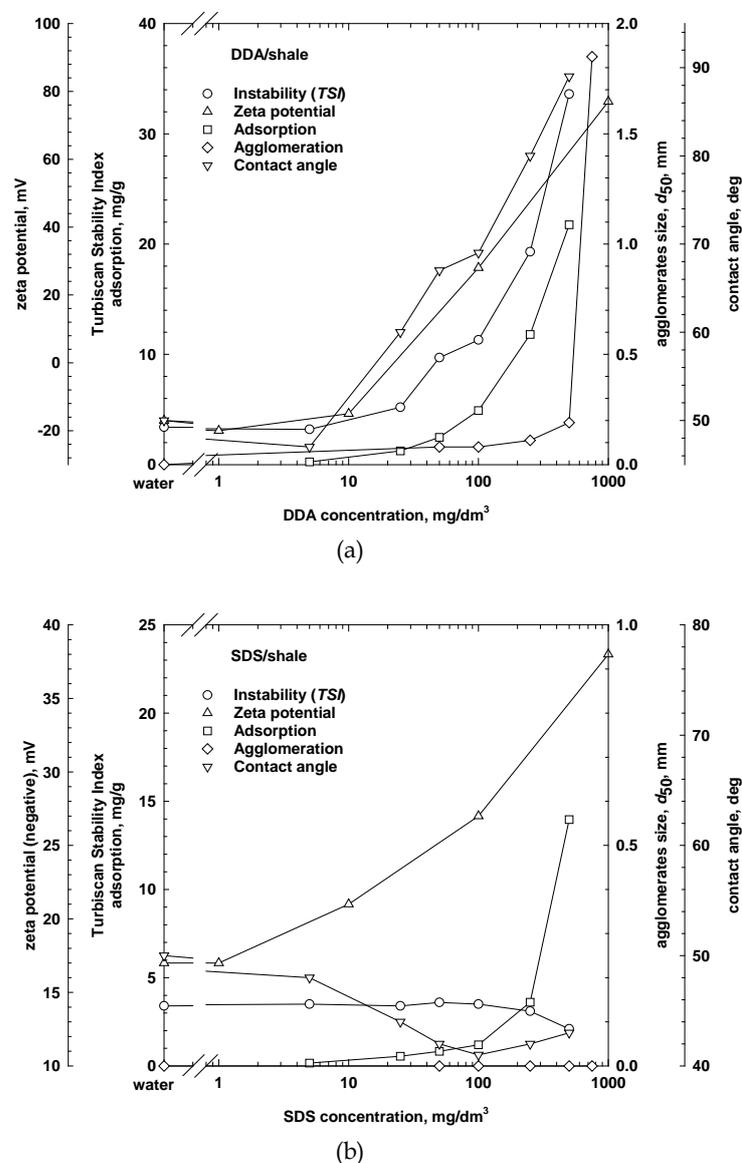
Fig. 2. Zeta potential, instability, adsorption, agglomeration and contact angle for metal-bearing shale as function of (a) DDA and (b) SDS concentration
