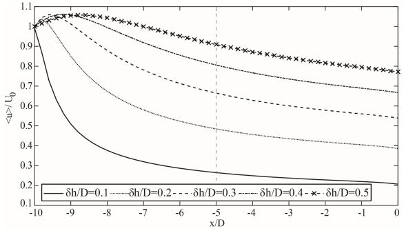
**Figure 4.** Streamwise velocity  $\langle u \rangle / U_0$  distribution along the horizontal extension in the symmetry plane and at different distances  $\delta h/D$  away from the cylinder surface. The resultes are from the v6h10 configuration. The vertical dashed line at x/D = -5 indicates the location where the 5D extension of the v6h5 configuration would have stopped.
