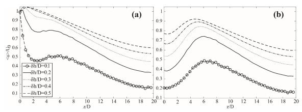
**Figure 7**.  $\langle u \rangle / U_0$  along the concentric quarter-rings  $\delta h/D = 0.1$ , 0.2, 0.3, 0.4, 0.5 away from the surface (in upstream direction) of the curved cylinder in the symmetry plane. (a) v6h0 configuration; (b) v6h10 configuration.
