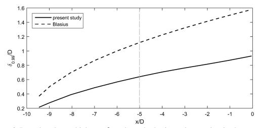
**Figure 6**. Boundary layer thickness  $\delta_{0.99}$  along the horizontal extension in the symmetry plane for configuration v6h10. The vertical dashed line at x/D = 5 indicates the location where a v6h5 configuration would have stopped.
