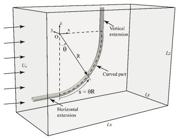
Figure 1. Sketch of the geometry of the concave curved cylinder and the computational domain. The uniform inflow  $U_0$  is from the left.
