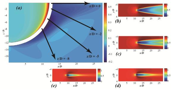
**Figure 3.** Flow fields for configuration v0h0. (a) Pressure distribution in the symmetry plane, *i.e.* the (*x*,*z*)-plane at y/D = 0; (b)-(e) Streamwise velocity contour plots at four different (*x*,*y*)-planes whose locations are z/D = 0, -2, -5, and -8, respectively.
