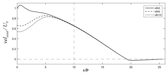
**Figure 9**. The axial velocity along the curved cylinder (including the 6D vertical extension), taken at  $\delta h/D = 0.3$  away from the cylinder surface.
