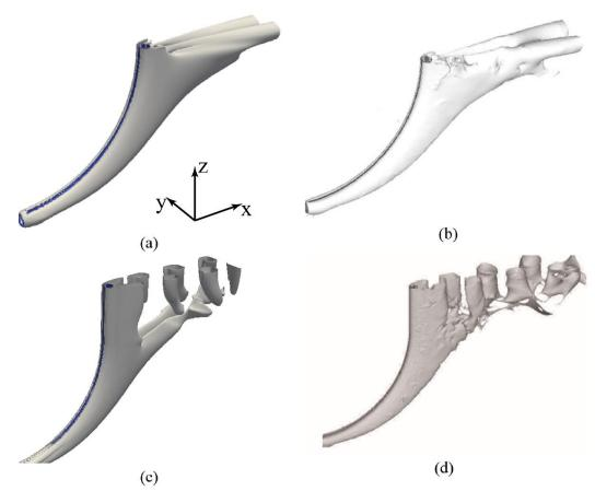
**Figure 2.** Qualitative comparisons of computed vortical structures and those reported in the literature<sup>[3]</sup>. (a) and (b) are v0h0 configuration, (c) and (d) are v6h0 configuration. (a) and (c) are from current study, while (b) and (d) are from Miliou et al.<sup>[3]</sup>. All plots show the iso-surface of  $\lambda_2 = -0.01$ . Note that the coordinate system in (a) just indicates the directions, but not location of the origin.
