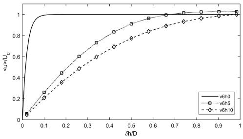
**Figure 5**. Boundary layer velocity profiles at position x/D = 0 in the symmetry plane for all configurations. The profile for the *v6h0* configuration is that defined by equation (1), whereas the two other profiles demonstrate how the boundary layer develops along the horizontal extension before it meets the curved part of the cylinder at x/D=0.
