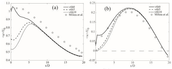
**Figure 8.** (a)  $\langle u \rangle / U_0$  along the curved cylinder at  $\delta h/D = 0.3$  away from the cylinder surface for the three different configurations; (b) same as (a) but for  $\langle w \rangle / U_0$ .
