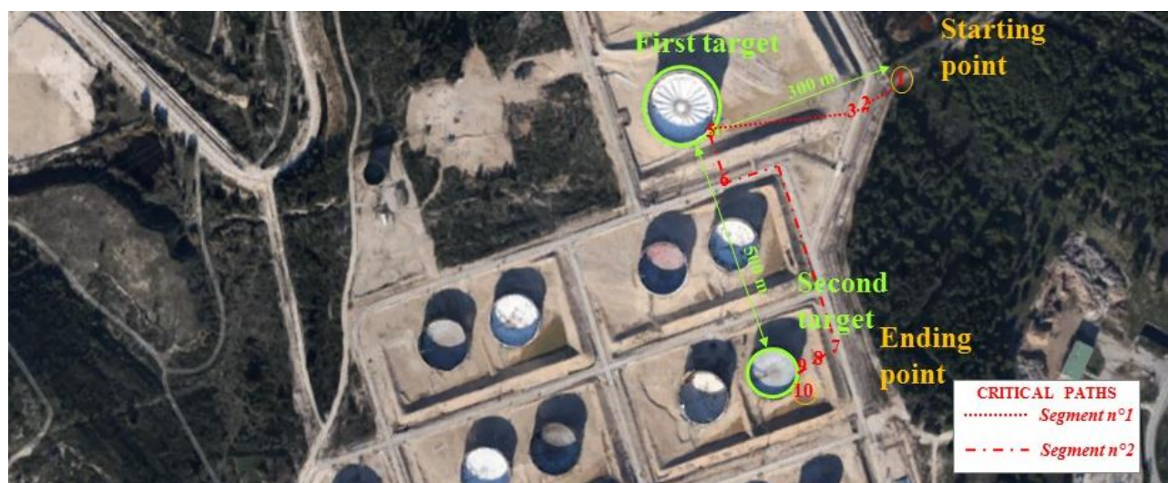
Fig. 2. Layout of a reference installation considered in the case study, with adversary starting point, sabotage targets and critical adversary paths, divided into two segments. Segment n°1 connects the starting point with the first target. Segment n°2 connects the first target with the second target. The ending point is the second target.
