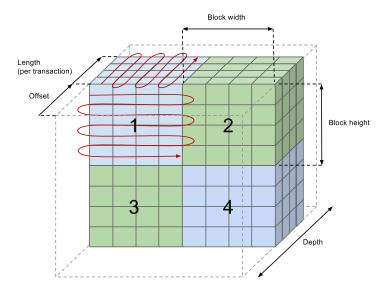
Figure 6: Processing order for a block-wise transfer in the CubeDMA
