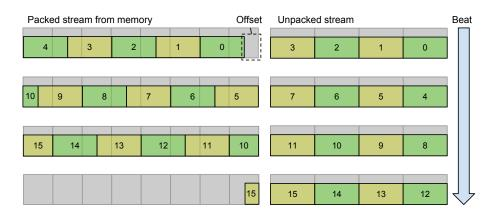
Figure 13: An example of packed data stream coming from memory and the resulting unpacked data stream
