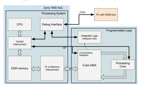
Figure 17: Overview of Zynq-7000 system for testing CubeDMA
