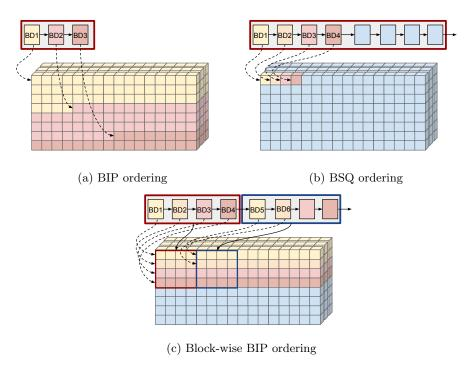
Figure 4: Creation of BD chain for different sample orderings
