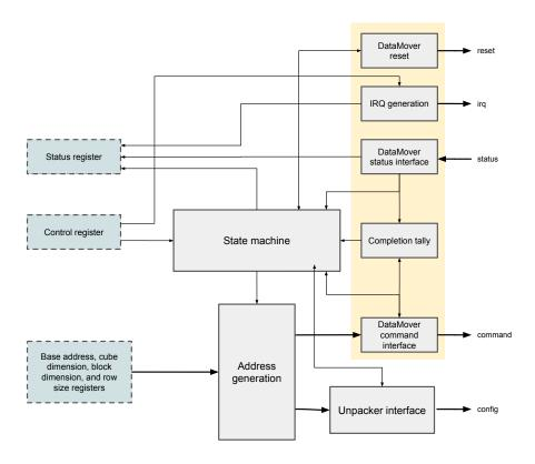
Figure 9: Architecture of the CubeDMA Controller module
