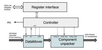
Figure 7: Architecture of the CubeDMA MM2S channel
