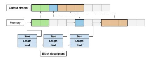
Figure 3: Scatter-gather transfer using a chain of block descriptors
