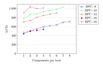
Figure 18: LUT usage for different BPC as a function of  $N_{\rm comp}$
