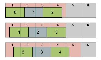
Figure 12: Number of bytes required to transfer three 10-bit components starting at various offsets
