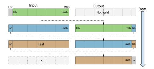
Figure 15: Behavior of the offset shifter
