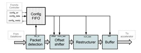
Figure 14: The Component unpacker module
