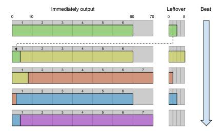
Figure 16: Example of a five-cycle restructuring process for 10-bit components and 64-bit input stream
