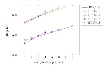
Figure 19: Register usage for different BPC as a function of  $N_{\rm comp}$
