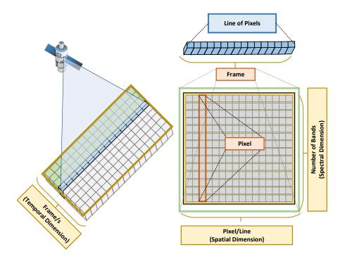
Figure 1: Hyperspectral cube acquisition process
