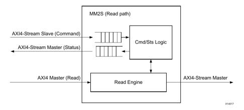
Figure 5: Overview of the DataMover core [15]
