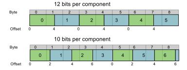
Figure 11: Component address, byte address and offset
