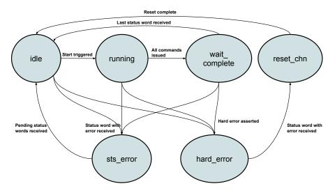
Figure 10: The state transition diagram for the State machine unit in the Controller
