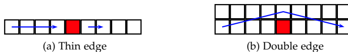
Figure 7.2: A single impermeable cell can pose problems for the localization assumption when interpolating pressure values
