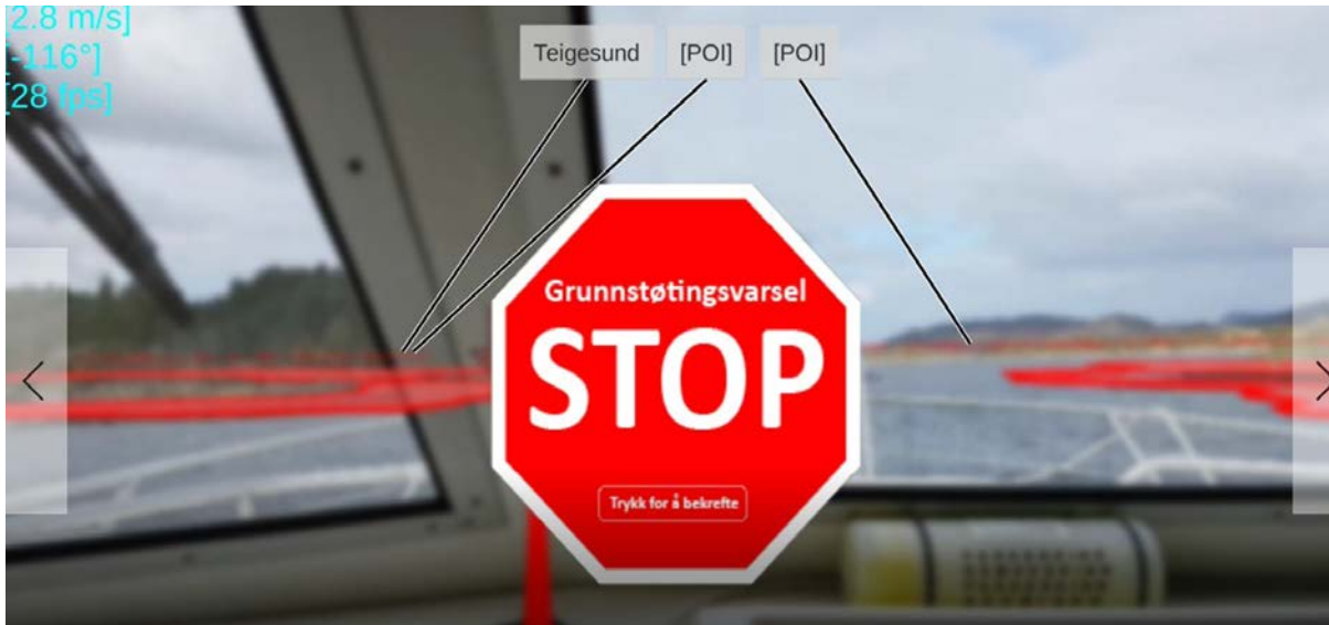
Figure 6. Screen dump from the Galaxy test phone. The grounding alarm has been triggered with both an aural and a visible alarm.
