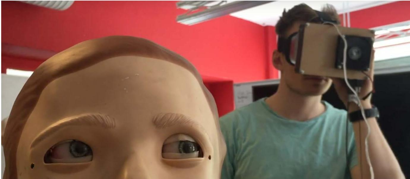
**Figure 1:** The operator (right) sees the live viewpoint of the mannequin (left) and directly controls the movement, incl. blinking, of the robotic eyes by the means of eye-tracking algorithms that are translated into according servo movements.
