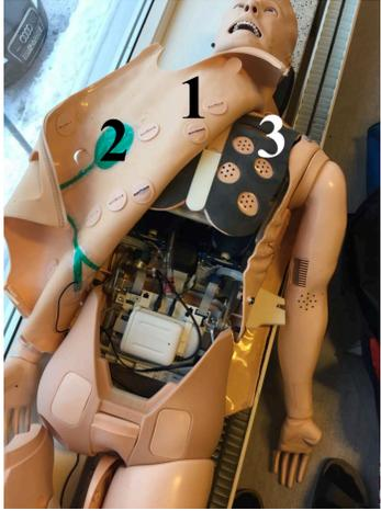
**Figure 2:** A high-end medical training mannequin, showing some of the interactive functionalities. 1) RFID chips in the skin enable location-specific, simulated ultrasound images. 2) The green patch is used for simulated defibrillation. 3) The rib cage contains speakers that provide simulated heart-beats or lung related sounds when listening with a stethoscope.
