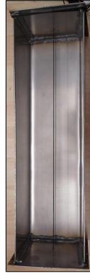
Figure 1. Upper image: schematical image of the experimental setup. Lower image: photo of the steel mold built to hold the epoxy during the experiment. The black thread visualizes the position of the optical fiber. The thread was replaced by the optical fiber before epoxy was cast into the container.
