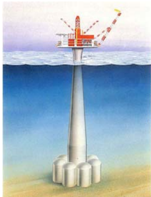
FIGURE 8. THE DRAUGEN PLATFORM: A ROBUST STATICALLY DETERMINATE (NON-REDUNDANT) REINFORCED CONCRETE STRUCTURE IN VIEW OF SHIP IMPACTS AND DROPPED OBJECTS. COURTESY: NORWEGIAN CONTRACTORS
