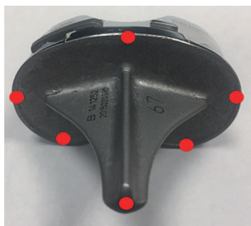
Figure 2. Fictive points of the tibial implant (the posterior fictive point is hidden behind the stem).
