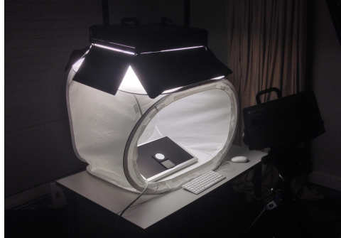
Figure 1: The setup was measured using a Konica Minolta CS-2000 Spectroradiometer (Ltd, 2018) at the viewing distance of 70cm.
