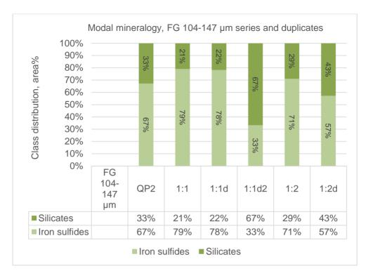
Figure 6. Modal mineralogy of samples from the FG 104-147 µm fraction and duplicate samples.
