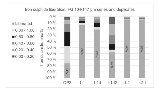
Figure 7. Iron sulfide liberation of samples from the FG104-147  $\mu$ m fraction and duplicate samples of 1:1 and 1:2.
