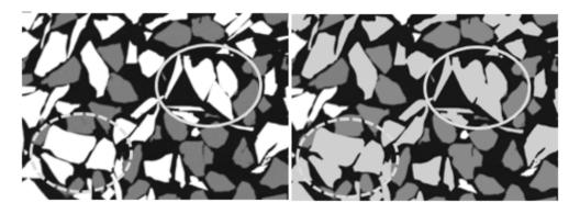
**Figure 1.** Examples of touching particles. BSE image (left) and binary image of reference sample QP 104-147  $\mu$ m. Dark particles=quartz, Light particles=iron sulfide. The grains in the solid circle are adjacent iron sulfides grains, interpreted as one particle. Grains in dotted circle are adjacent quartz and iron sulfides interpreted as one particle.
