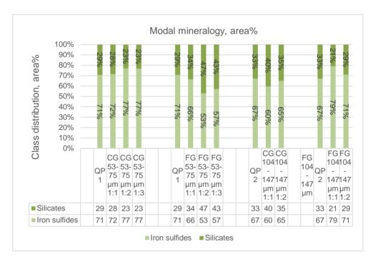
Figure 3. Modal mineralogy from PTA analysis. The areal distribution of silicates and iron sulfides.
