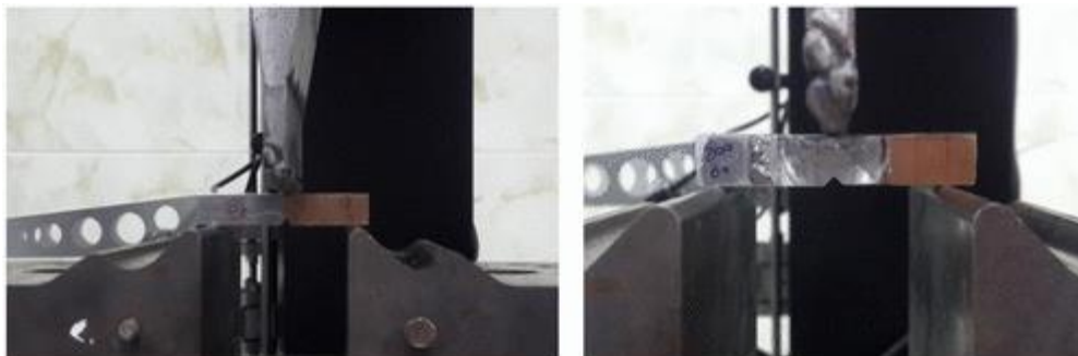
Figure 3. Typical test setup for three-point bend loading of notched Al–Cu bimetal.
