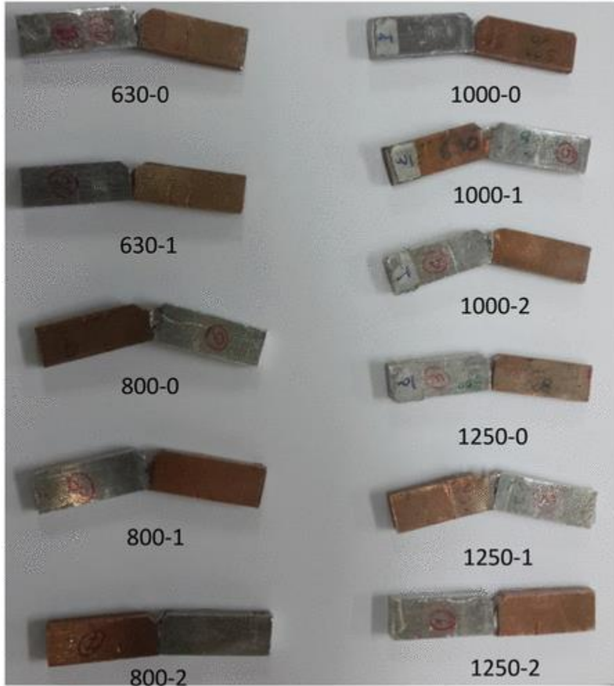
Figure 5. Fracture trajectory obtained for some of the tested Al–Cu bimetals.
