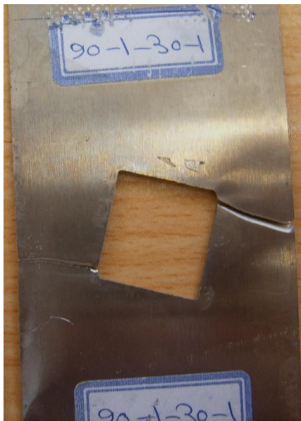
(b) Large plastic deformations at the ligament
