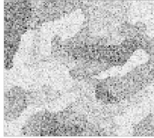
(b) Observed picture: Independent Gaussian noise with \sigma = 1.0 added to each of the nodes in the underlying picture.
