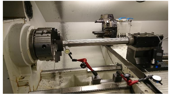
Fig. 3. Vibration-damped boring bar with strain gages in the test lathe.
