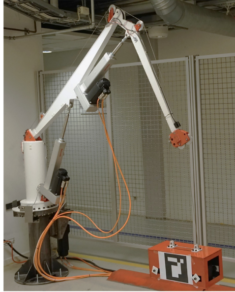
Fig. 1. A down-scaled version of a knuckle boom crane.
