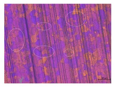
Figure 47: LOM image illustrating grain boundary attacks, encircled in white. 10x magnification. The scale bar is 50  $\mu$ m.
