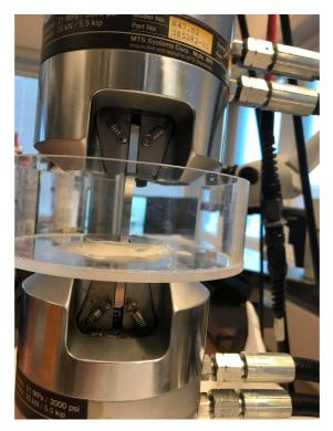
Figure 27: Image of sample mounted to chamber in fatigue machine.
