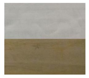
**Figure 2.** Visual inspection of an epoxy resin showing discoloration due to hygrothermal aging. **Top**: initial (blueish grey); **bottom**: redried after conditioning (yellow).
