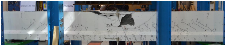
Fig. 4 Figure of the failure for beam 4 (LWAC65_20_100).
