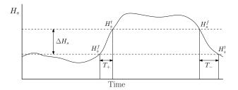
Figure 5: Analysis procedure for determination of transition periods of  $H_s$
