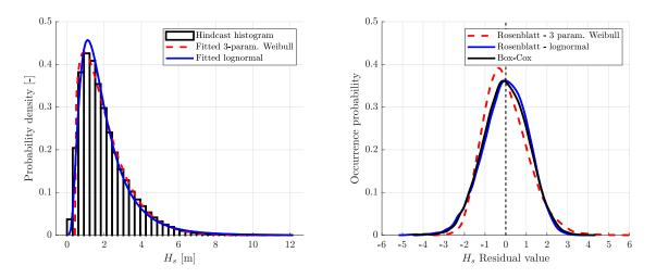
Figure 3: Distribution fit for hindcast wave data (left) and residual distribution plot (right)
