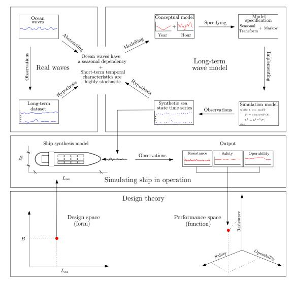
Figure 1: The stages of wave modelling and its connection to ship performance evaluation during design, exemplified by Markov model. (Top part of figure adapted and modified from [27])
