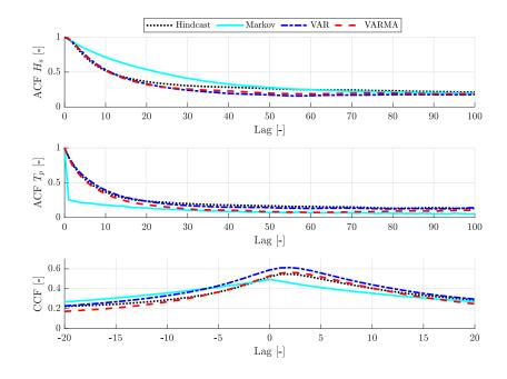
Figure 11: Autocorrelation function (ACF) and cross-correlation function (CCF) for hindcast and model  $H_s$  and  $T_p$  time series
