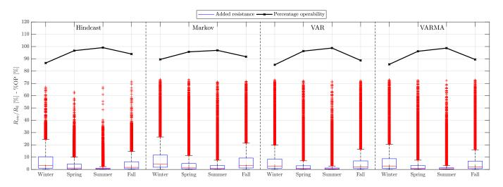
Figure 12: Added resistance estimates for speeds 15-20 knots according to attainable speed curve.
