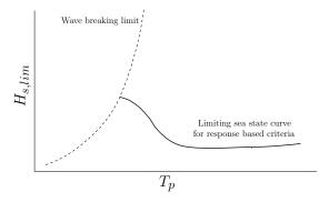
Figure 7: Limiting  $H_s$  as a function of  $T_p$  for response based criteria
