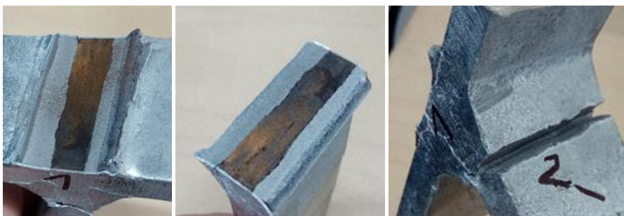
Figure 3. This specimen is an example of both the failure mechanism for the tested detail, Geometry 1: it failed for initiation at the weld root with propagation through the weld (left and center), while, contemporarily, a second crack initiated and propagated at the weld toe on the other side (right).
