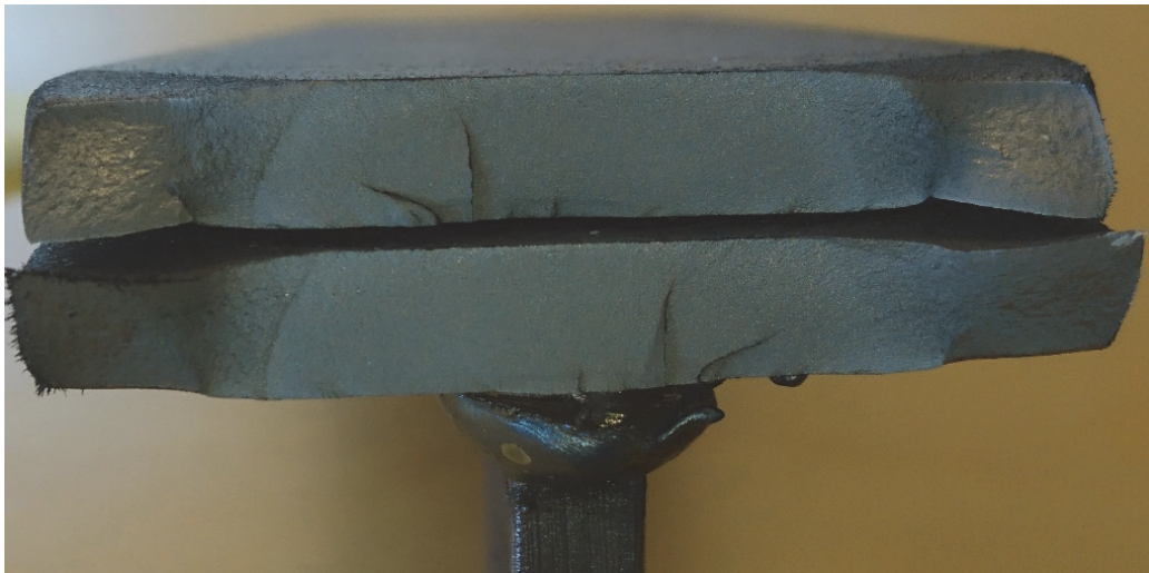
Figure 6: Detail of the fracture surface. The same type of surface characterizes all the failures in the experimental campaign.
