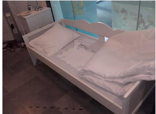
**FIGURE 1** | Bed equipped with a visible flat pressure sensitive sensor.
