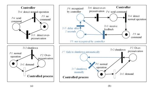
Figure 6-5 SPN models for (a) adequate control (b) two potential loss scenarios
