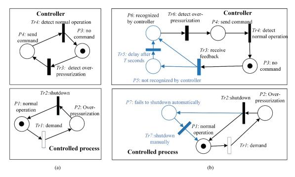
Figure 4 Mapping control structure into SPN: (a) adequate control and (b) two potential loss scenarios
