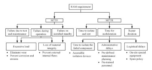
Figure 9-2 Factors to be considered in allocation model of subsea design
