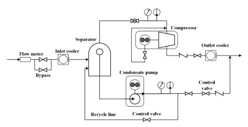
Figure 2-2 A simplified schematic of a subsea processing system
