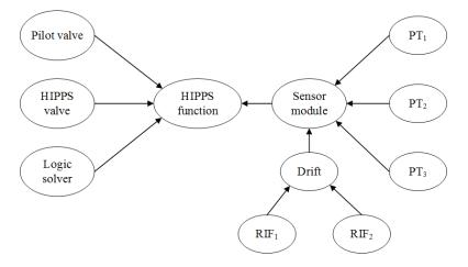
Figure 7-5 BN model that incorporates the effect of sensor drift
