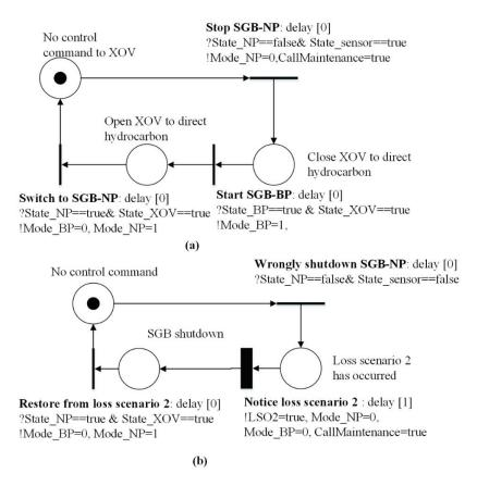
Figure 6-8 Mapping safe scenario and loss scenario into SPN model
