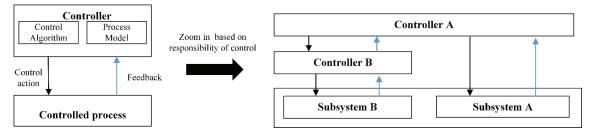
Figure 2 Example feedback control loop
