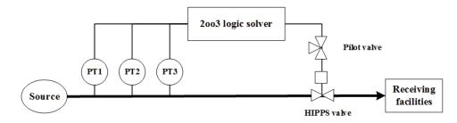
Figure 7-2 The schematic of HIPPS functions
