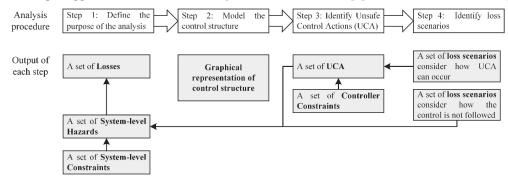
Figure 1 the framework of STPA and its output
