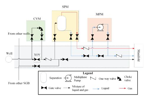
Figure 6-6 System schematic drawing of SGB
