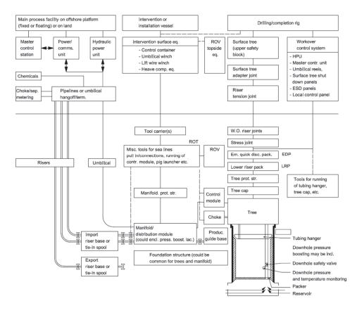
Figure 2-1 Subsea production system, adopted from ISO 13628-1 [17]
