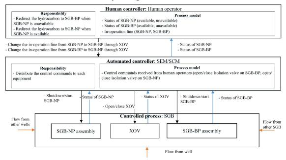
Figure 6 High-level control structure of SGB
