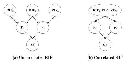
Figure 7-1 BN models of RIFs, component failure and system failure rate
