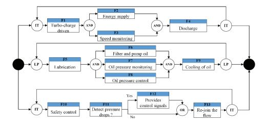
Figure 5-4 FFBD for subsea gas compression
