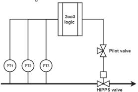
Figure 2. schematic of HIPPS functions
