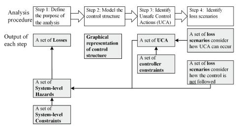
Figure 6-2 The framework of STPA and its output
