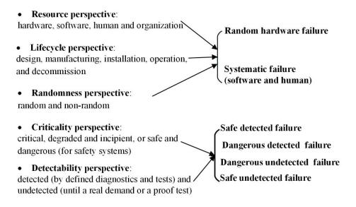
Figure 6-1 Commonly-used perspectives for failure classification
