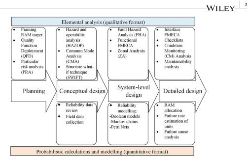
FIGURE 1 Mapping RAM methods in design process
