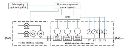
FIGURE 5 Subsea fiscal oil export metering system<sup>44</sup>
