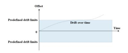
Figure 7-3 Sensor drift over time
