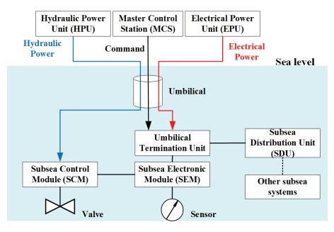
Figure 2-3 A simplified schematic for multiplex electrohydraulic control system
