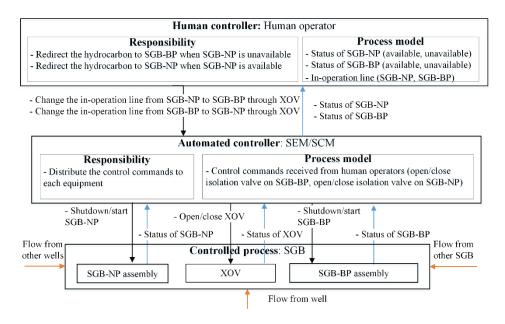
Figure 6-7 High-level control structure for SGB
