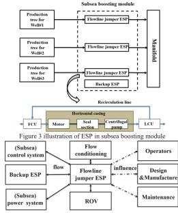
Figure 4 Flow line jumper ESP and its environment
