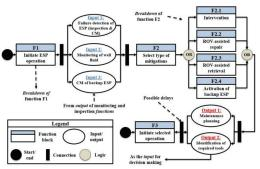
Figure 5 function model for fault response during operation
