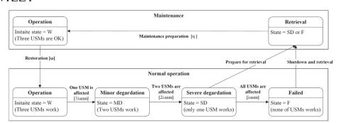
FIGURE 7 State diagram for USM assembly
