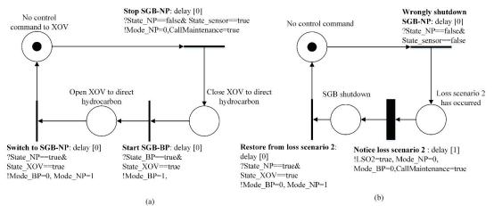
Figure 7 Mapping safe scenario and loss scenario 2 into SPN models
