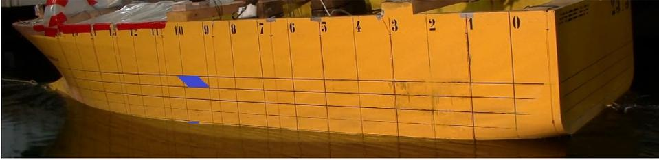
*Figure 6.48: Sinkage and trim of the model in test C551.*
