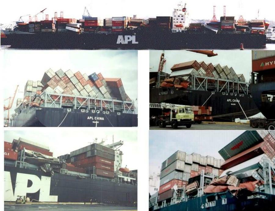
Figure 1.1: The APL China Incident [Images from [www.cargolaw.com](http://www.cargolaw.com)].
