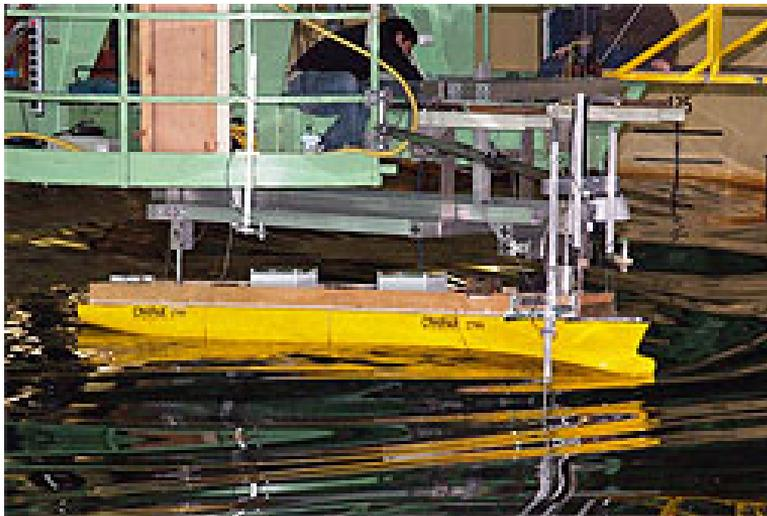
Figure 5.3: C11 post-Panamax container ship model and the experimental set-up [38].
