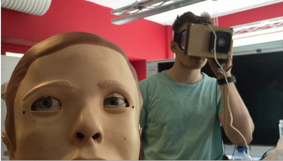
Figure 1.9: In order to increase the possibilities and levels of interaction with medical training mannequins, TrollLABS developed a set of eyes that is remotely controlled by tracking the eyes of an external observer who has the viewpoint of the mannequin itself.
