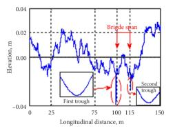
Figure 4. Trough and road profile with troughs
