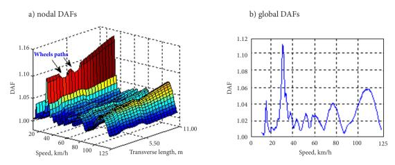
Figure 10. DAF-speed pattern for plate model due to a series of 38 moving point loads travelling with an eccentricity with respect to the bridge centreline
