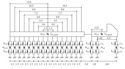
Figure 1. Side view of 19-axle vehicle (all dimensions in meters)
