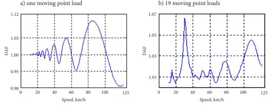
Figure 5. DAF-speed pattern due to
