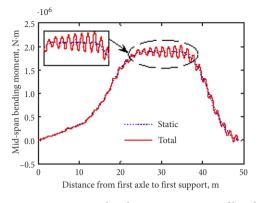
Figure 6. Maximum total and static component of bending moment at mid-span versus location of the first axle
