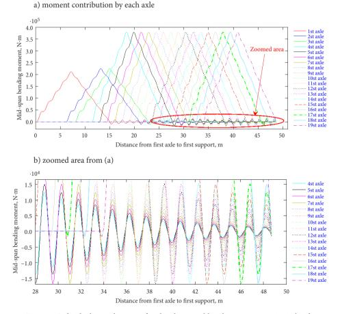
Figure 7. Individual contributions of each axle to total bending moment at 30.24 km/h
