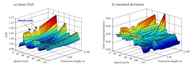
Figure 11. DAF-speed for plate model due to long vehicle on class A profile
