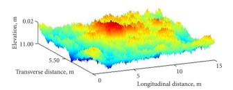
Figure 3. Bridge surface based on the class B road profile
