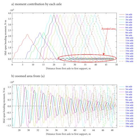
Figure 8. Individual contributions of each axle to total bending moment at 39.96 km/h
