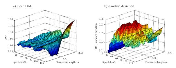
Figure 12. DAF-speed for plate model due to the 5-axle truck on class A profile
