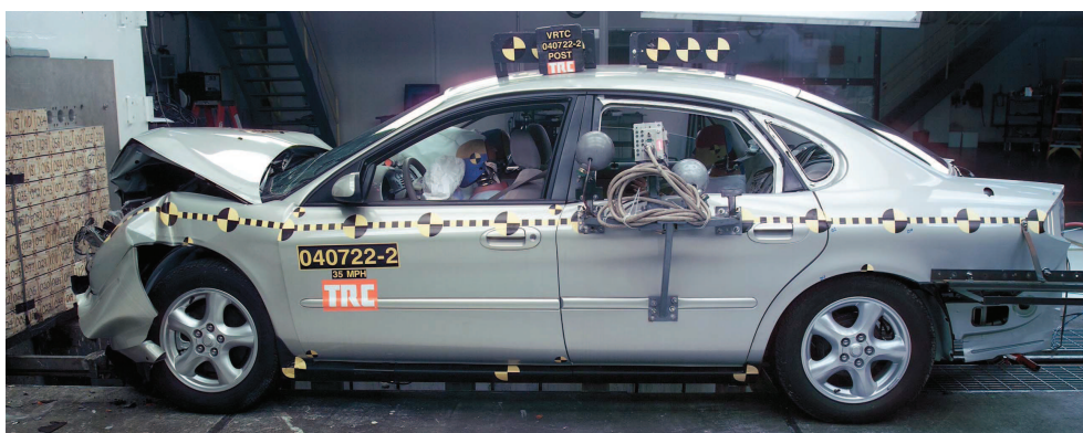
Figure 1. Full-scale crash test of a Ford Taurus (2004 model) at 56 km/h [35].
