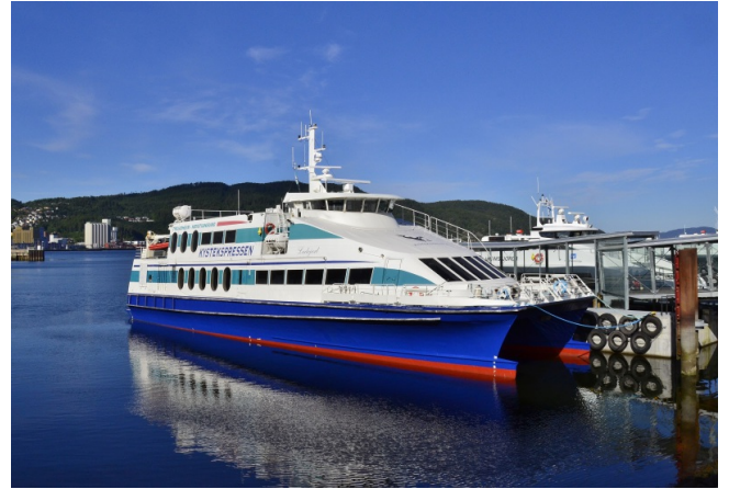
Figure 5: The passenger ship MS LADEJARL (gross tonnage 490 t, length 38 m, breadth 10 m)
