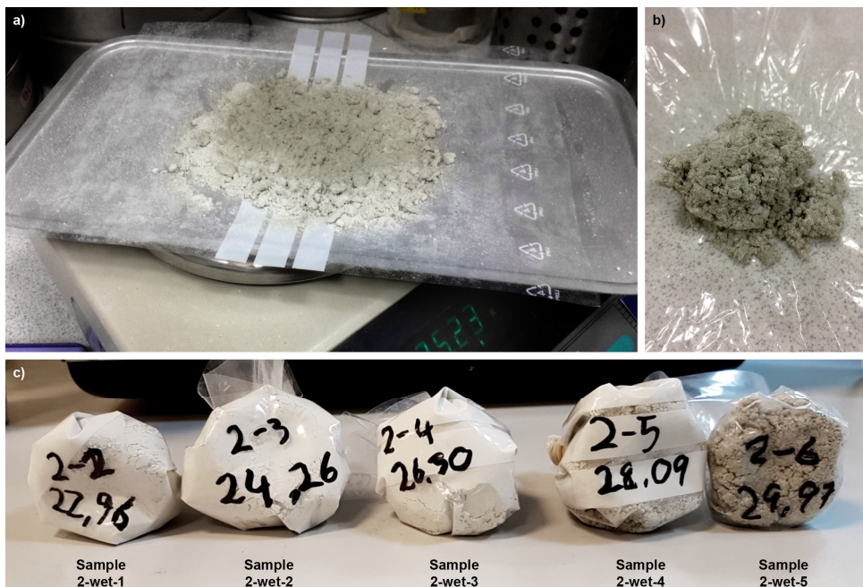
Fig. 6 Sample preparation. a) Adding water on sample 2-wet-5 with a spray bottle. The material was mixed with a spatula while the water was added. b) Sample 2-wet-5 before applying the rubber band. A spatula was used to collect all material and water in the middle of the plastic sheet. c) Sample series 2. The total weight was marked on the bag for easy control of any water leaving or entering the material. Bag marked 2-2 is later called 2-wet-1, 2-3 is called 2-wet-2 and so on
