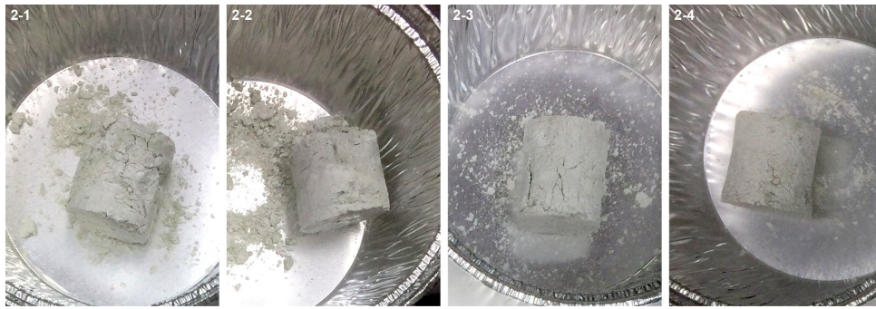
Fig. 5 Samples from E39 Svevatjørn – Rådal after drying and extraction from brass cylinder
