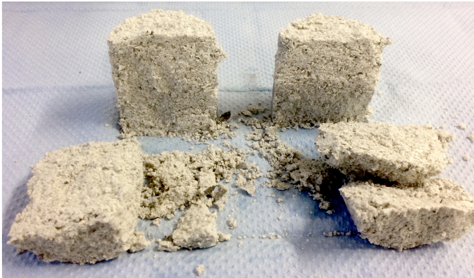
Fig. 9 Test sample 2-8 split after testing to check quality of water addition. In the case of dry zones they were easy to detect
