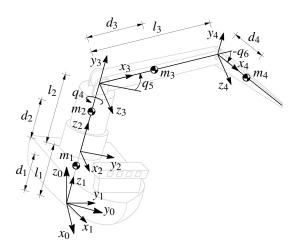
Fig. 4. A crane/vessel system consists of four bodies: a vessel, a crane king, an inner boom and an outer boom.
