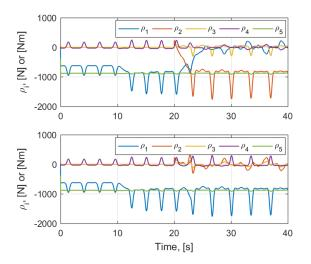
Fig. 7. The constraint forces and moments between the crane and the vessel are given in the coordinates of Frame 1 (on the top) and in the coordinates of Frame 2 (in the bottom).
