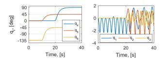
Fig. 6. The crane joint variables are regulated according to the motion sequence given in Fig. 5. The vessel is initialized at its origin. The motion of the vessel is excited by the crane motion.
