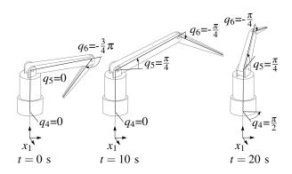
Fig. 5. Positions of the crane throughout the simulation represent the sequence of crane positions during a typical hoisting operation.
