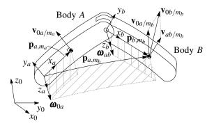
Fig. 1. An ordered couple of vectors of angular velocity and linear velocity constitute a twist. The hatched area spanned by the angular velocity and the distance vector is the magnitude of the linear velocity. Twists referenced to the same point and expressed in the coordinates of the same frame can be summed up.
