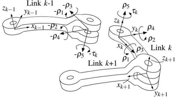
Fig. 3. For bringing noncontributing constraint forces to evidence, we imagine that Link  $k$  can lose the contact with Link  $k-1$  and start moving with some additional velocities in the direction of the unknown constraint forces. Note that the gap between the links is only drawn for the demonstration purposes.
