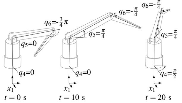
Fig. 5. Positions of the crane throughout the simulation represent the sequence of crane positions during a typical hoisting operation.
