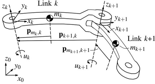
Fig. 2. A crane can be generalized as a robotic manipulator arm, where the links are connected by pivot joints with one actuated rotational degree of freedom in each joint.
