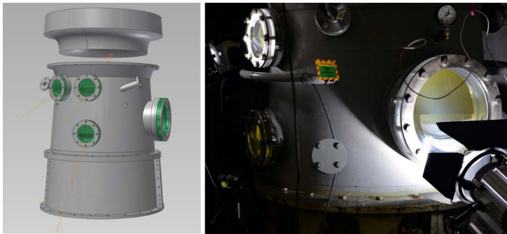
Figure 2. (a) Outline of the acrylic-glass windows mounted on the draft tube with the adequate vision angle to see the blades; (b) photograph showing the flow visualization tests.
