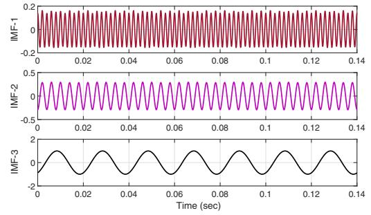
Fig. 4. Extracted IMF by EMD
