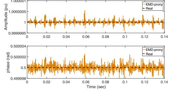
Fig. 5. Amplitude and phase estimates by EMD-Prony ( $L=3$ )
