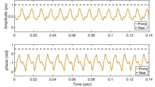
Fig. 6. Amplitude and phase estimates by traditional Prony ( $L=1$ )
